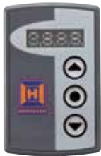
External control element for FUE-1 For easy operation and programming, can be placed independent of the control, same control buttons as on the control, 4 × 7-segment display
