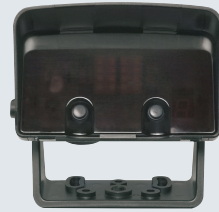
Radar movement detector MWD Fast and targeted automatic door opening, directional recognition, max. fitting height 7 m, fitting in cold store possible to max. - 22 °C, IP 65
