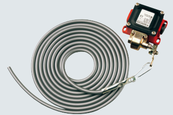
Pull switch with plastic pull cord Horizontal or vertical fitting possible, aluminium die-cast housing, IP 65, cord length 4 m
