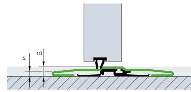
The stainless steel threshold is 10 mm high at the centre and 5 mm at the edges. We provide a reinforced threshold rail of approx. 13 mm for doors from 5510 mm width or for doors with real glass from 4510 mm width. For doors with real glass in the wicket door area already starting at 4510 mm door width!
