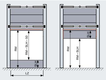
When the coupled door is opened (right figure), the bottom section with the catwalk remains in the top part of the door opening.
