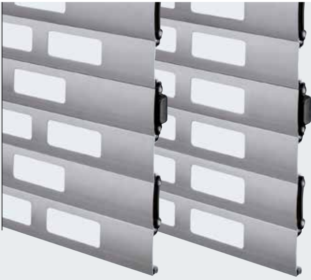
HG 75, aluminium The extruded aluminium profiles are available in a powder-coated surface finish. The 100 × 40 mm square holes can be provided in a straight or offset arrangement.
